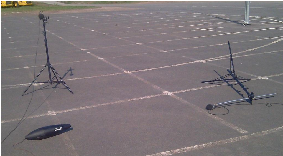
Figure 11 Setup for calibrating sound source - on the picture sound source and two microphones
