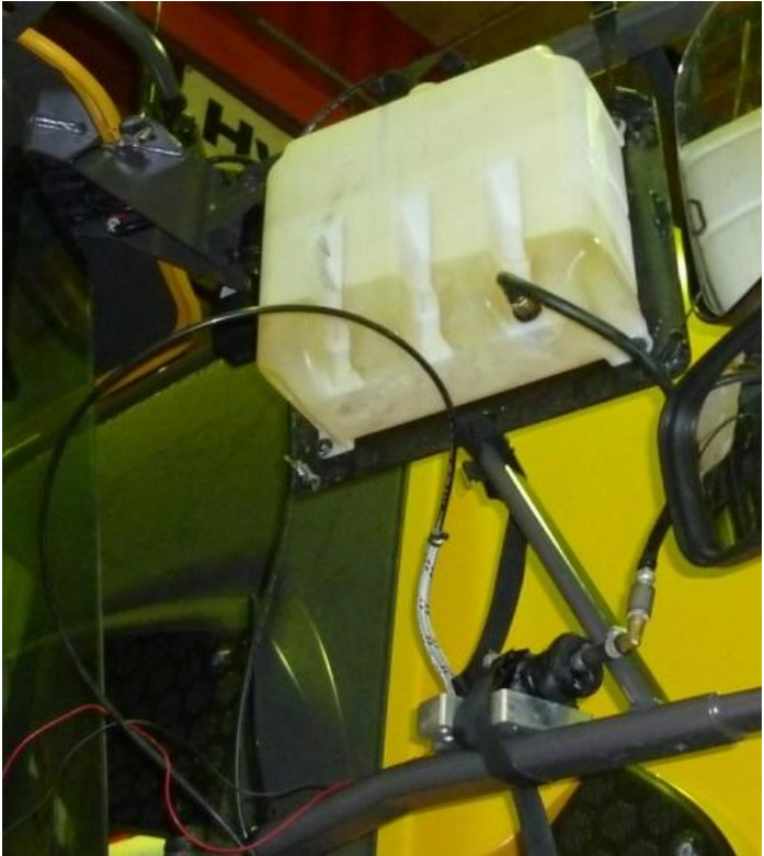
Figure 4 Oil tank with pump
