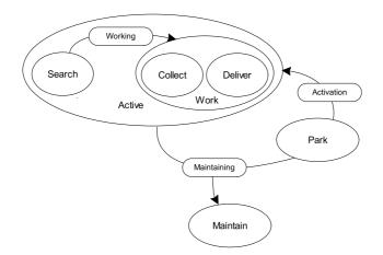
Fig. 3. The role diagram of the AGV.
