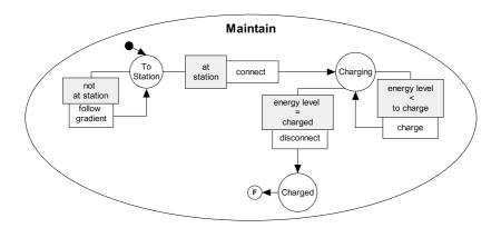
Fig. 4. Action diagram of the Maintain role.
