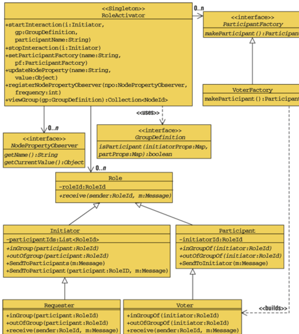
Figure 3. UML diagram of ObjectPlaces' API. RoleActivator is the main access point to ObjectPlaces' services, offering methods to start and stop interaction sessions. Roles, such as Requester and Voter, should be implemented as subclasses of either Initiator or Participant.
