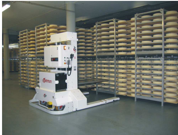
Figure 5.1: An AGV at work in a cheese factory
